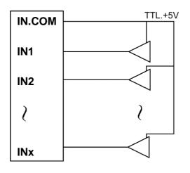
**TTL/CMOS signal Input**
