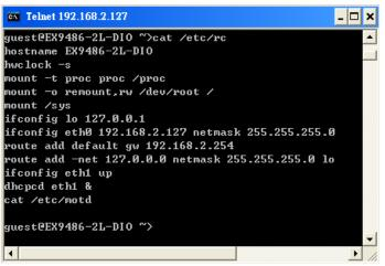
To configure the IP address, Netmask and Gateway setting, please modify /disk/etc/rc as following:
